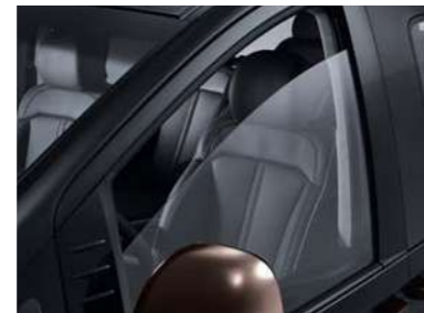
1st-row double-laminated soundproof glass
